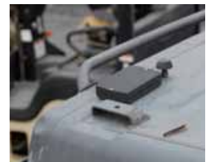
Tracker installed on shovel cab roof.
