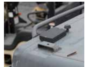
Tracker installed on shovel cab roof.
