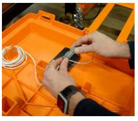
**4 LAST STEP** - Reconnect the gray waterproof connector that links the white power cord to the tracker
