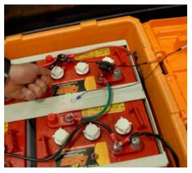
Disconnect tracker wires from the battery terminals
