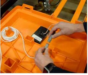
Disconnect the gray waterproof connector between the battery wires and the tracker
