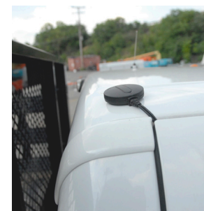
GOOD ANTENNA INSTALLATION LOCATIONS are on roofs, with constant access to the sky. Out of harm's way.
