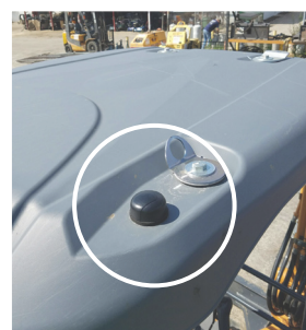
GOOD ANTENNA INSTALLATION LOCATIONS are on roofs, with constant access to the sky. Out of harm's way.
