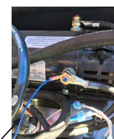
Run 3rd Wire (blue) along back of battery drawer and connect with ring terminal
